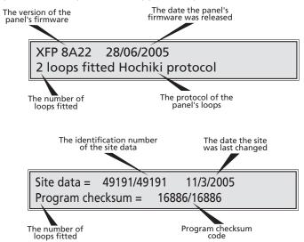
Matching site data codes, i.e. 49191/49191 and program checksum codes, i.e. 16886/16886, show that the panel is functioning correctly. Mis-matched numbers, i.e. 49191/40286, indicate that the panel's memory may be corrupt. After five seconds the panel will return to the Engineering Functions submenu.
