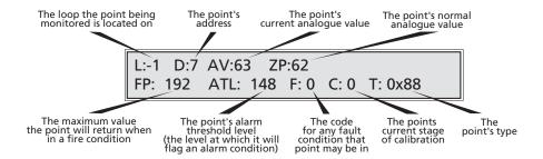
To return to the Engineer Functions submenu press the Escape ◀ button.
