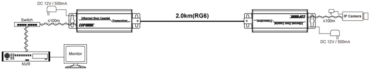
◆Application Diagram 2: Star Two Cameras EoC Transmission System
