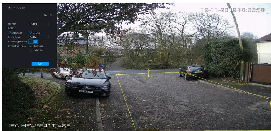
Rules can be created using the left mouse button to draw Tripwire or Intrusion lines on the image in the area of interest. In the top left window, the direction of travel can also be selected. Once the rule is configured, click **Ok**
