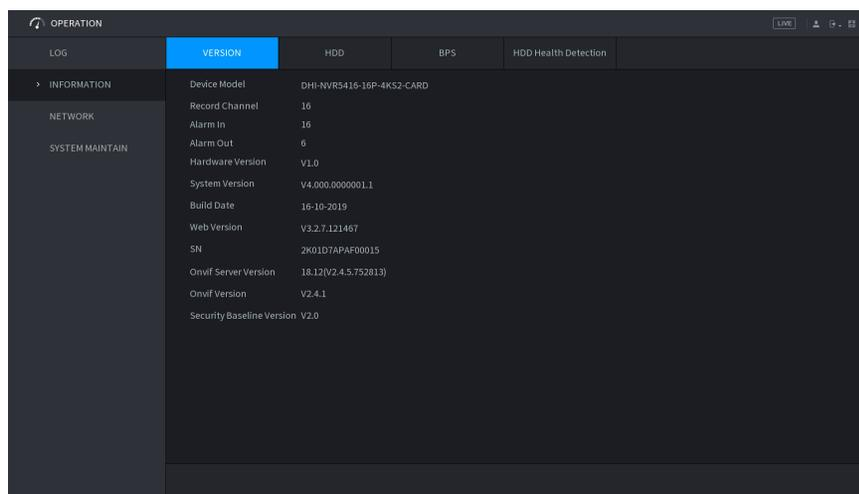
NVR/DVR firmware is often updated to introduce better optimisation and add new features. To check the firmware currently installed on the system go to **Menu > Operation > Information**
