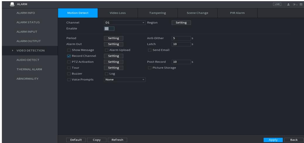
To enable motion detection select the **Enable** box.
