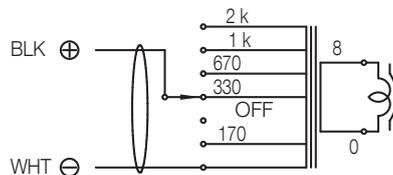
(Transformer connection when the speaker is supplied from the factory)
