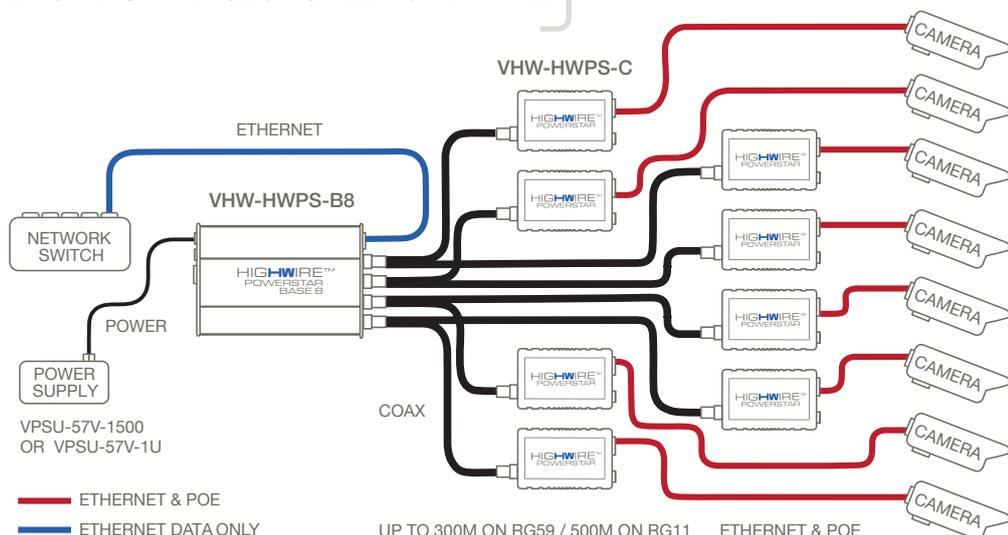
RACKMOUNT ETHERNET AND POWER OVER COAX SOLUTION
